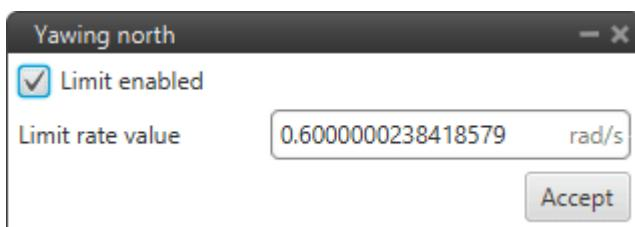
With this block it is desired that the aircraft maintains the yaw to the north (angle 0°).
