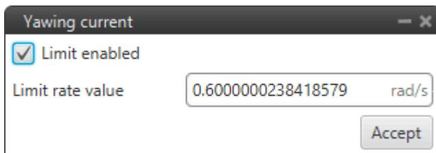
In addition, a **limit rate value** of 0.6 rad/s has been defined to control the speed at which the aircraft yaws in the guidance of this phase.
